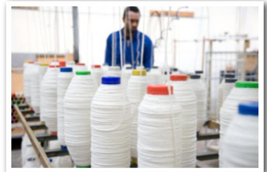
**Radford Yarn Technologies** process natural New Zealand wool into a range of high-end felted yarns for carpet and rug manufacture. Heat from the boiler is required for their felting plant, and their yarn drier.
